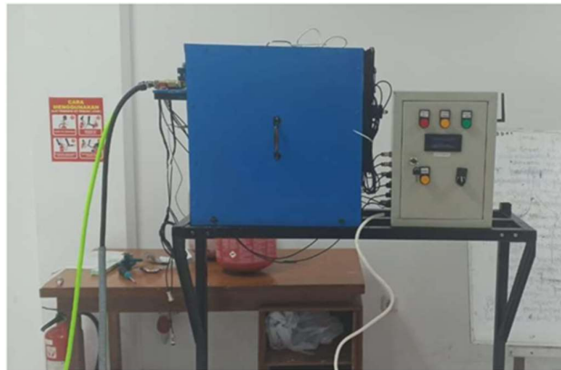
Fig. 4. Hardware implementation, the blue box is the gas reactor and the white box is the electric panel.
