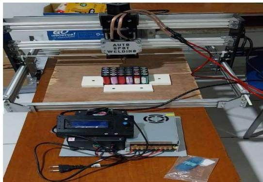
Gambar 5. Rangkaian mesin CNC spot welding baterai lithium 18650
